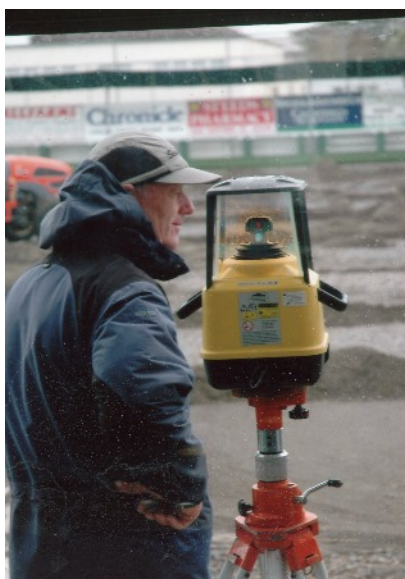
The laser leveller on the bank was linked to the receiver on the tractor.
